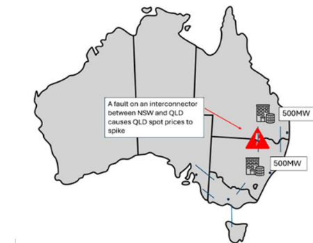
Figure 2: Virtual interconnector capacity and automated inter-regional arbitrage using a flexible data centre portfolio
